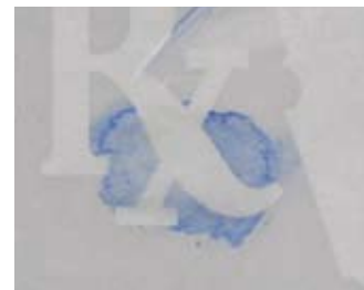
Solvents used to remove ink causes a visually evident "blooming" effect of ink.
